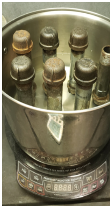
Figure 1. Metal vessels immersed in distilled water in a stainless-steel cookpot on a Precision™ induction cooktop.
