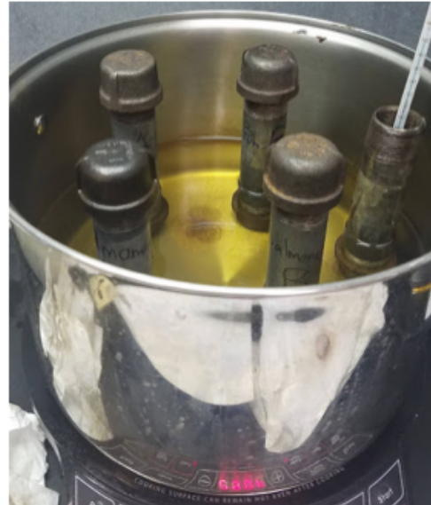
Figure 3. Metal vessels immersed in peanut oil in a stainless-steel cookpot on a Precision™ induction cooktop.
