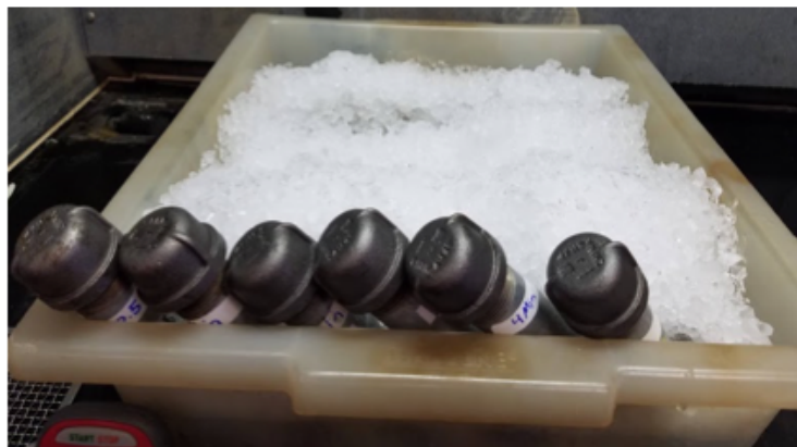
Figure 2. Metal vessels in ice-laden cold water (0°C) to halt heat transfer
